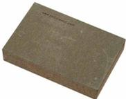
**BetonWood N** The Betonwood cement bonded particle board, high density ( $1350 \text{ Kg/m}^3$ ), realized with Portland cement conglomerate and debarked Pine wood fiber. Thermo-dynamics characteristics: thermal conductivity coefficient  $\lambda=0,26 \text{ W/mK}$ , specific heat  $c=1,88 \text{ KJ/Kg K}$ , coefficient of resistance to vapor penetration  $\mu=22,6$  and fire resistant class A2-fl-s1, according to the standard EN 13501-1.
