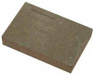
**BetonWood N** The BetonWood N cement bonded particle boards, with high density (1350 Kg/m<sup>3</sup>), made of Portland-type cement conglomerate and debarked Pine wood fiber. These panels have the following termo-dynamics characteristics: thermal conductivity coefficient  $\lambda=0,26$  W/mK, specific heat  $c=1,88$  KJ/Kg K, coefficient of resistance to vapor penetration  $\mu=22,6$  and reaction to fire class A2-fl-s1, according to the standard EN 13501-1.
