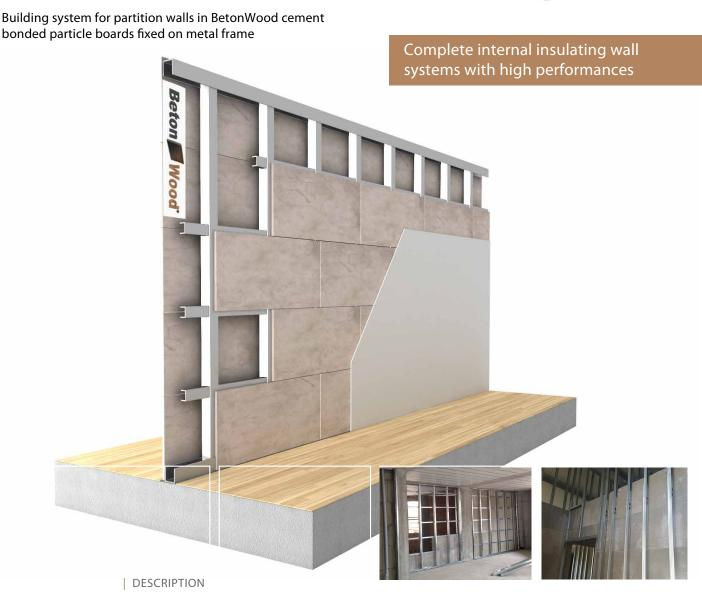
The complete building system for high performances internal wall Partition wall Betonwood on metal is easy and quick to install, guarantees maximum comfort and durability over time, with the international ETA certification.
