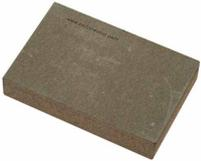
**BetonWood** The BetonWood cement bonded particle boards, with high density (1350 Kg/m<sup>3</sup>), made of Portland-type cement conglomerate and debarked Pine wood fiber. These panels have the following termo-dynamics characteristics: thermal conductivity coefficient  $\lambda=0,26$  W/mK, specific heat  $c=1,88$  KJ/Kg K, coefficient of resistance to vapor penetration  $\mu=22,6$  and reaction to fire class A2-fl-s1, according to the standard EN 13501-1.
