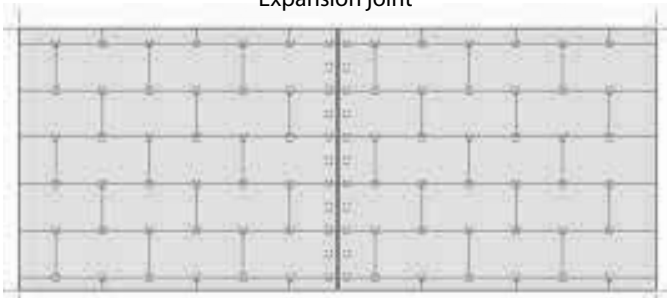
Placement of an expansion joint with position of the supports (interaxis 30 cm) - FOR ENVIRONMENTS OVER 40 m 2
